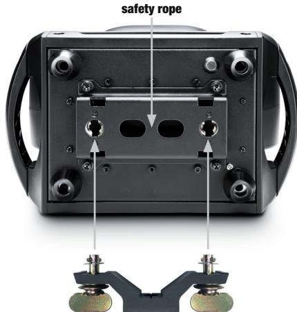
**EN** Thanks to the integrated rubber feet, the spotlight can be placed in a suitable location on the stage floor etc. Mounting on a truss is performed using the supplied omega mounting bracket (please use only the original mounting bracket); secure the device with a suitable safety rope to the space provided (please fasten the safety rope prior to installing the omega mounting bracket). Important Notice: Overhead installation should only be carried out by trained personnel.
